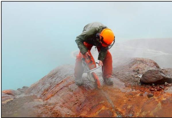
Photo 7: Cutting first side of a channel sample at Big Bulk.
