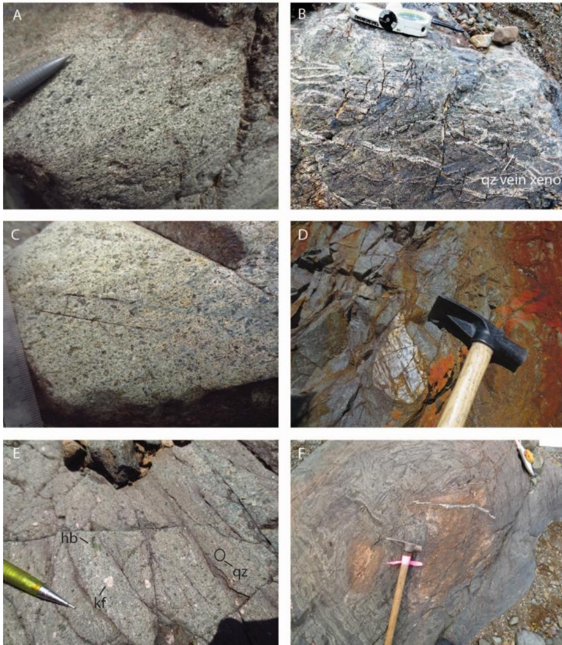
Figure 4. Kinskuch plutonic rock phases of intrusion. A: Phase 1 diorite is green, medium-grained, crowded, magnetite-hornblende- diorite porphyry overprinted by pervasive propylitic calcite-epidote-chlorite-pyrite-chalcopryrite alteration. 475063 E, 6166399 N (photo ID 3082). B: Phase 2 synmineral hornblende diorite contains quartz-chalcopryrite vein xenoliths that are cut by quartz-chalcopryrite sheeted quartz veins and pervasive chlorite-quartz-magnetite alteration; 476094 E, 6167052 N (photo ID 3271). C: Phase 3 green, medium-grained, crowded, hornblende diorite porphyry is overprinted by quartz-sericite-pyrite-chlorite (QSPC) alteration; 477715 E, 6166876 N (photo ID 3455). D: Xenolith clast of sheeted quartz veins (SQV, Phase 2) contained within Phase 3 hornblende diorite porphyry overprinted by quartz-chlorite-pyrite alteration; 477926 E, 6166916 N (photo ID 3346). E: Phase 4 monzonite is green, medium-grained, with 1-5 mm pink euhedral K-feldspar and green hornblende phenocrysts in equigranular hornblende-quartz-K-feldspar-plagioclase groundmass; 476441 E, 6166597 N (photo ID 3692). F: Flowbanded contact zone of Phase 4 monzonite with internally stockworked Phase 3 hornblende diorite xenolith clasts, 476168 E, 6166722 N, (photo ID 3113).
